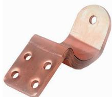
This copper foil flexible connection is constructed by stacking multiple layers of copper foil, with both ends pressure-welded.
